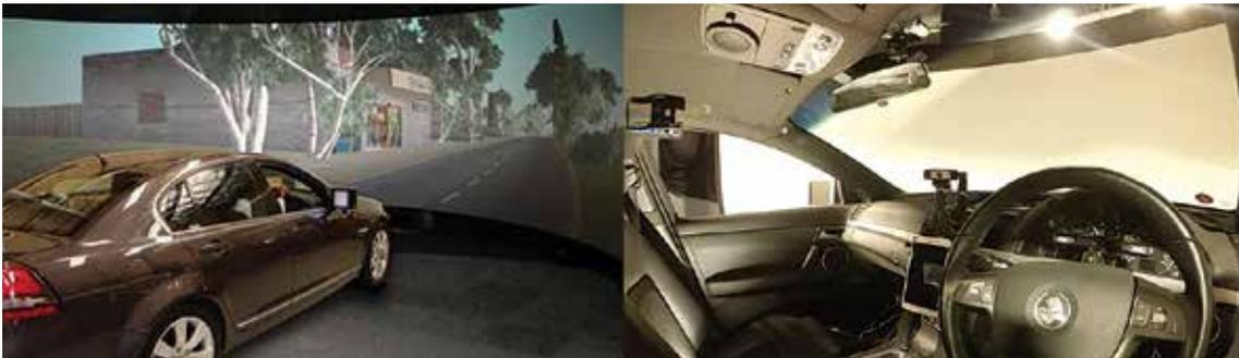
MUARC Advanced Driving Simulator (top) and integration with Seeing Machines' Driver Monitoring System (bottom)
